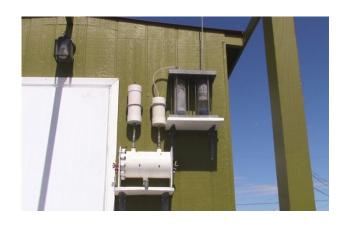
Hydrogen Wind Electrolyzer, Foam Traps & Double Bubbler
