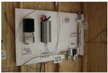
PV electronics and H2 purification system
