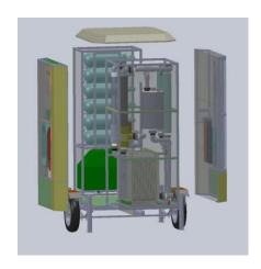
After several years of development and gallons of blood, sweat and tears, the Hysolgenics solar EL-5000 electrolyzer is finally producing hydrogen. The AHA has ordered one and it is now being mounted on a trailer for transport to Phoenix. It will produce about 1 cubic foot of H2 per minute. See it at work:
