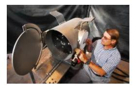
This mouth-full from Sandia National Lab uses a parabolic mirror to heat a chamber of water and nasty CO2 to 1500° C, producing hydrogen, oxygen and carbon monoxide, precursors to synthetic fuel. They say it could be ready for market in 15 to 20 years. If people keep up this sort of thing, we may never see that \$20 a gallon gasoline.
