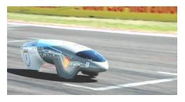
The PAC-Car II, built at the Swiss Federal Institute of Technology in Zurich, achieved 12,666 mpg using a hydrogen fuel cell and two small electric motors. (www.paccar.ethz.ch) Read all the details in "The World's Most Fuel Efficient Vehicle: Design and Development of The PAC-Car II." J. J. Santin and others, 2007. About \$64, 339 pages. Get an extra copy for Detroit.
